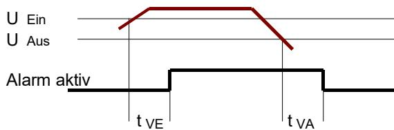
Note for high voltage relay: an alarm is set off when specific minimum, or better low voltages are reached. Low voltages are different for each relay type and do not correlate to programmable error voltages.
