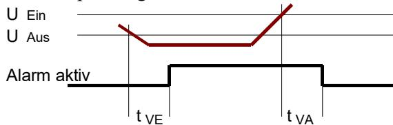
Note for low voltage relay: Relay R released means “Alarm Active.”
