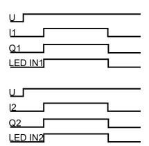
Triggering the input I1 switches on the output Q1 (e.g. electromagnet) immediately.
