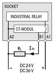
A freewheeling diode as surge suppressor is already integrated in the module. An additional, external coil suppression is not necessary.
