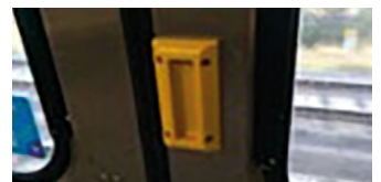
A new style door handle retrofitted to the Comeng trains, designed to make it harder to force the doors open
