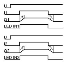
When triggering the input I1, the voltage on output Q1 will be raised to the nominal value linearly during the preset time slot. The motor is accelerated to defined speed.
